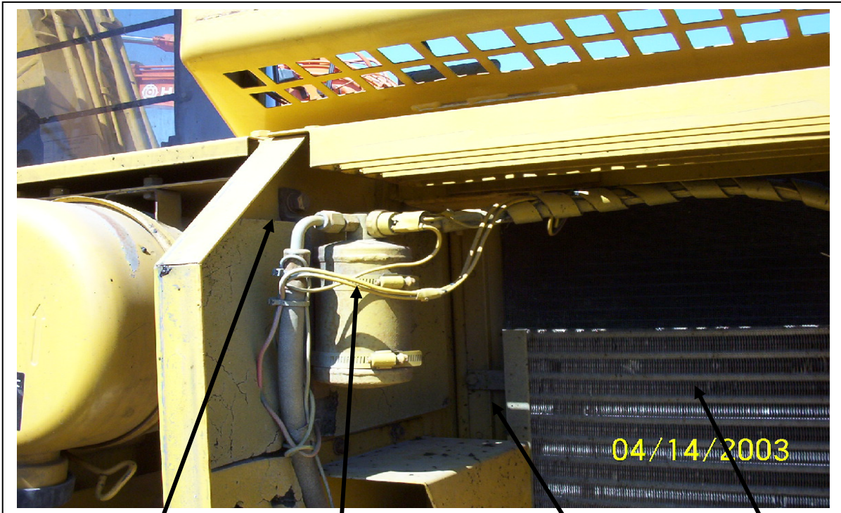
Drier bracket mount point
