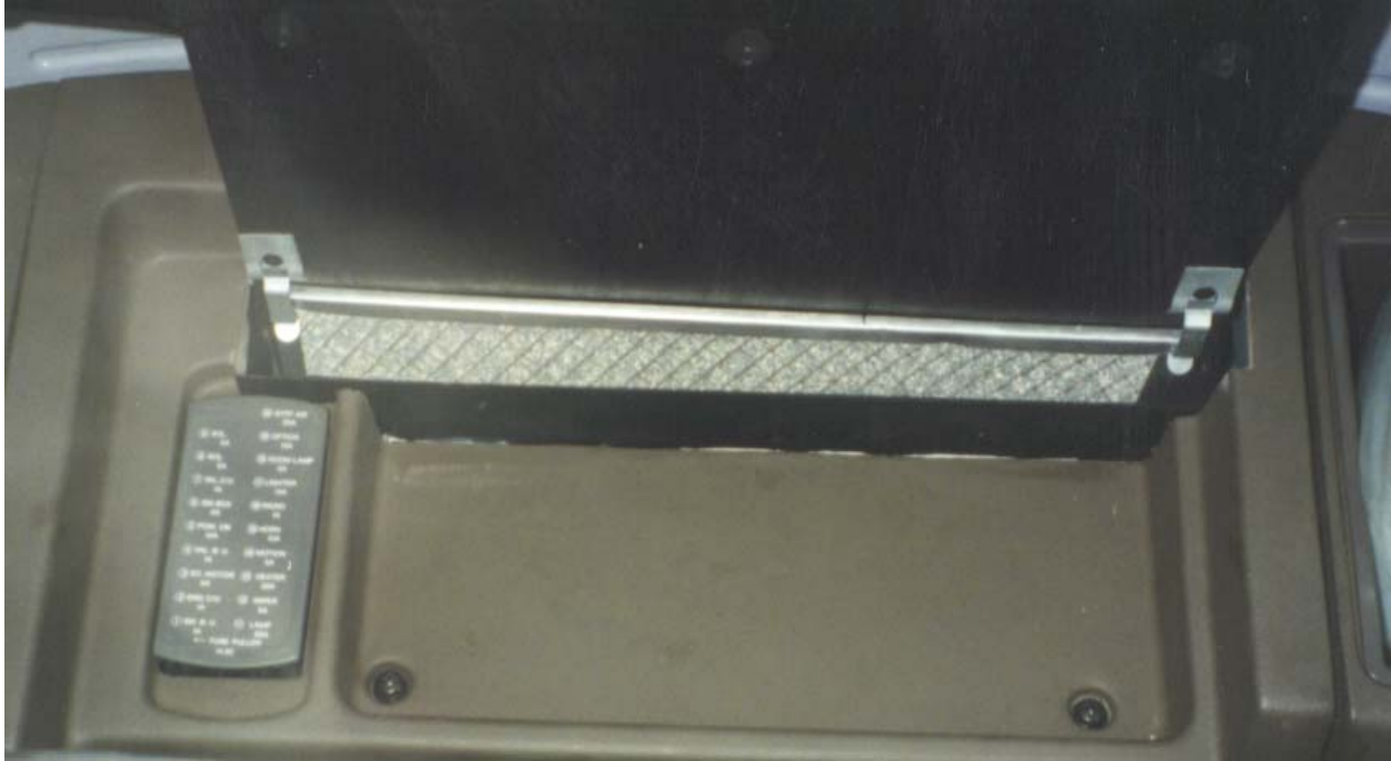
Bottom of evaporator showing cut-out in center trim panel.
