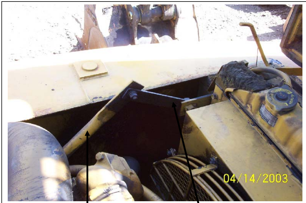
Radiator support bracket
